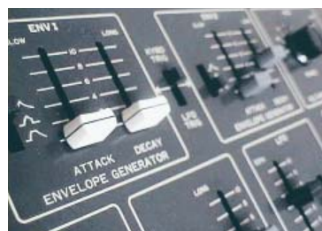
PUSHING THE ENVELOPE: Sliders are used for the Kawai Synthesizer 100-F's envelope generator section.
