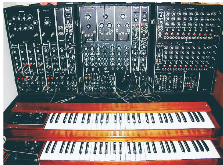
RING, RING, TELEPHONE RING: While it's easy to mistake this Moog modular system for a telephone operator's patch bay, it's actually a synthesiser.
