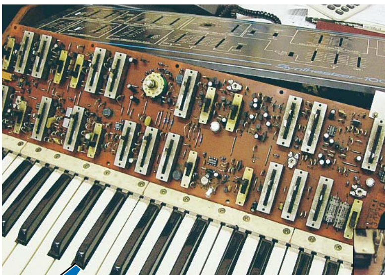
▲ EARLY ENGINEERING: This is what the interior of an analogue synth looks like – a simple, single VCO, sans memory, monophonic monster, a Kawai Synthesizer 100-F in this case. ▶ ANALOGUE PLAYGROUND: The interior of the Kawai Synthesizer-100F up close.
